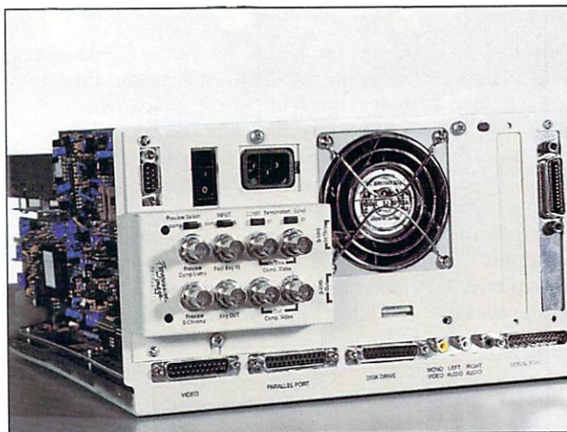
The SuperGen 2000s hardware includes the internal board and a breakout box that installs on the rear of the machine.
